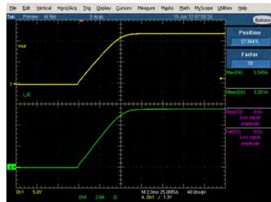
Figure 2. SS Vin=24V, Cref=1nF, CVdr=1μF, Cv3V=1μF, css=68nF, Io=5.5A
