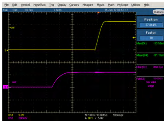
Figure 1. Vref and Vout start-Up Vin=48V Vo=12V
