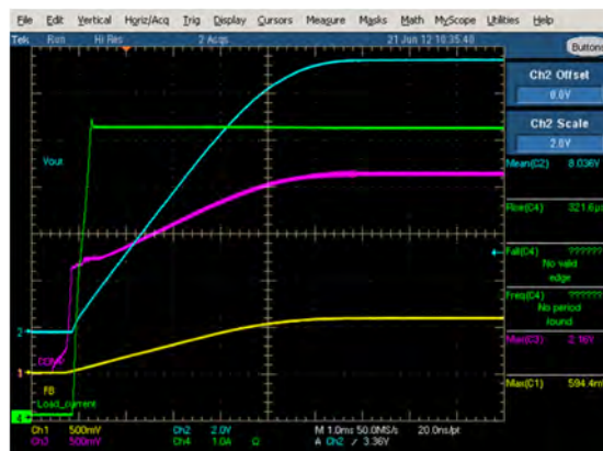
Figure 6. Detailed start-up operation, 24Vin, Vo=12V, 6A Ch1 (yellow): FB pin (negative input to the error amplifier), Ch2 (blue): Vout,
