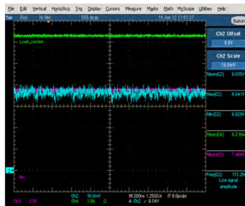
Figure 32. Ripple 8Vin Vo=6V, 6A 5MHz
