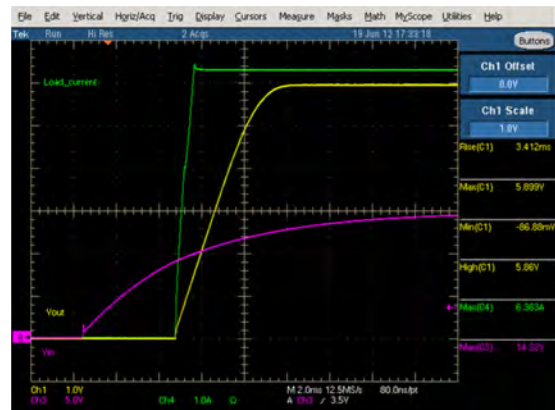
Figure 3. Start-up 15Vin Vo=5.8V, 6A, 5MHz
