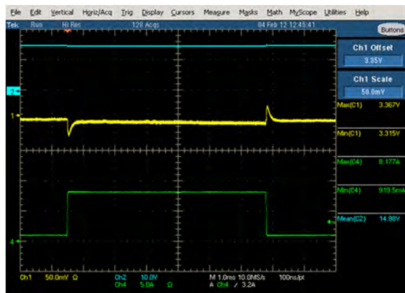
Figure 37. Transient step response Vin=15V, Vo=3.3V 2.2MHz 1-8A
