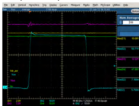
Figure 8. Switching node signals 24Vin, Vo=12V, 6A Ch1 (yellow): Vdrive_external, Ch2 (blue): switching node Ch3 (purple): Vout, Ch4 (green): Vin
